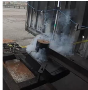
Figure 2. Image of Vapour Cloud produced from crush penetration of Li-ion battery cells. Taken from BESS Safety Alert 31/2021
